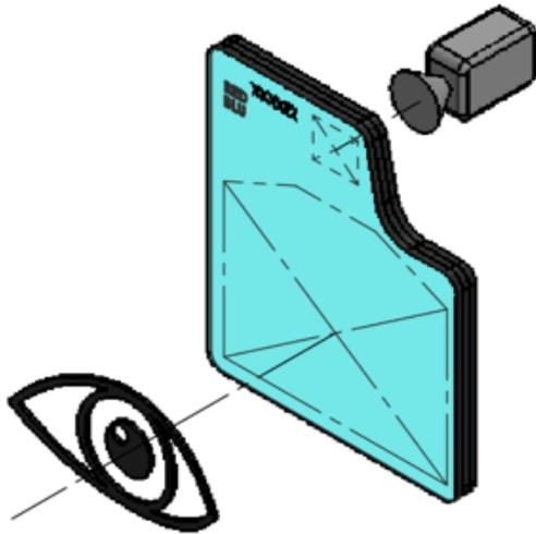
Figure 2 - Waveguide operation (Transmission mode)
