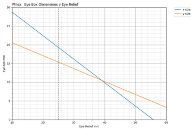
Figure 4 -Maximum eye motion box vs eye relief
