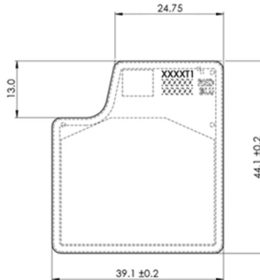
Figure 4 – Waveguide Dimensions
